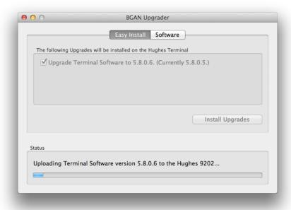
Figure 5: Sample screen for Normal Mode Upgrade in Progress Part 3 (Easy Install Pane): Uploading the New Software
